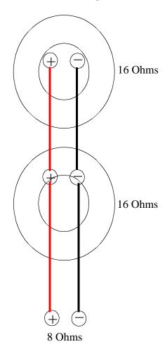
Two 16-Ohm speakers wired in parallel to yield a total load of 8 Ohms.
