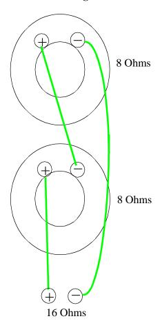
Two 8-Ohm speakers wired in series to yield a total load of 16 Ohms.
